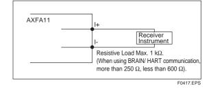
Figure 4.4.9 4 to 20 mA DC Output Connection
